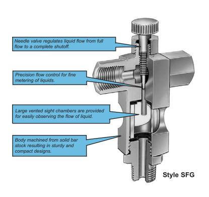
**SMALL SIGHT FEED VALVES** control the volume of liquid being dispensed while permitting visual observation of liquid flow. The valves are primarily used on gravity or pressure lubricating systems for bearing lubrication on machinery. Their use can be extended to any application requiring adjustable, visible, flow control. They are equipped with needle valve control that regulates liquid flow from full flow to a complete shutoff.
