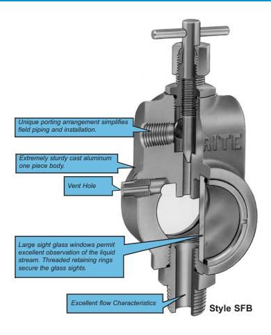
**UNIVERSAL PATTERN BULLS-EYE SIGHT FEED VALVES** allow visual observation of the liquid stream from a distance, with the volume of flow controlled by an adjustable needle valve. The Bulls-eye sight feed
